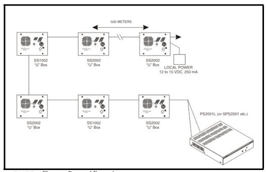
FIGURE 4. Phantom Powered Example
